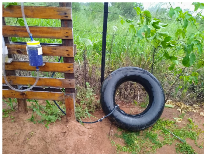
Figure 4 – Air chamber filled with biogas
