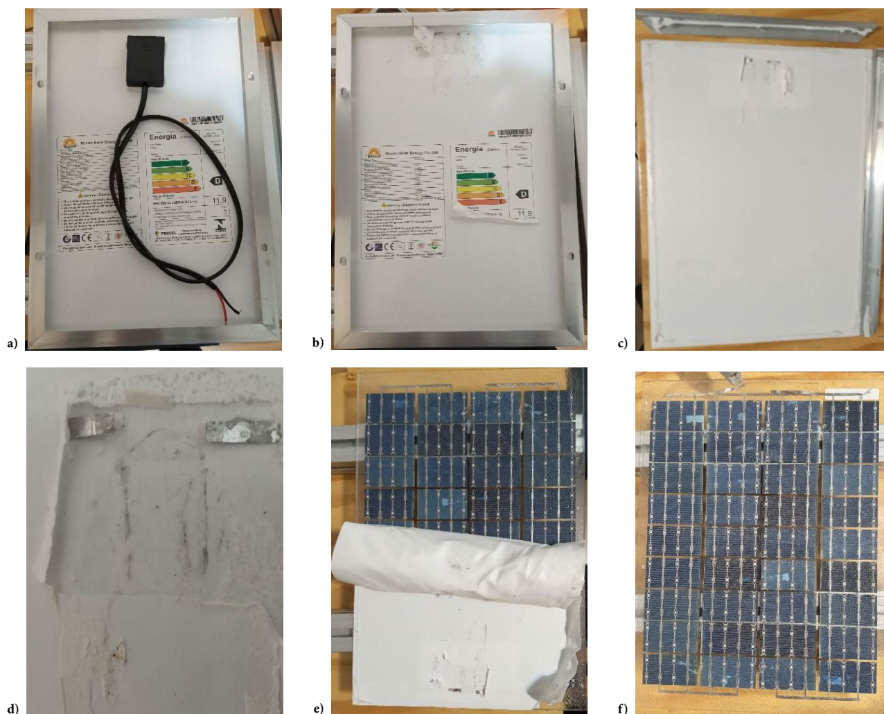
Figure 3 – Different stages of the disassembly of a solar panel. (a) Photovoltaic panel's back; (b) Photovoltaic panel's back without a junction box; (c) Photovoltaic panel's back without tags and frame; (d) Junction box contact detailing; (e) Panel's backside with the backsheet foil being removed; (f) Photovoltaic cells exposed before recovery with the assistance of a metal spatula and a heat gun.
