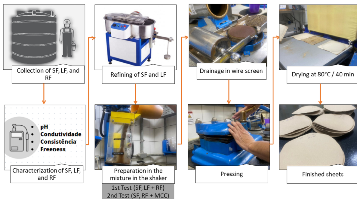
Figure 1 – Process stages for sheet formation.
