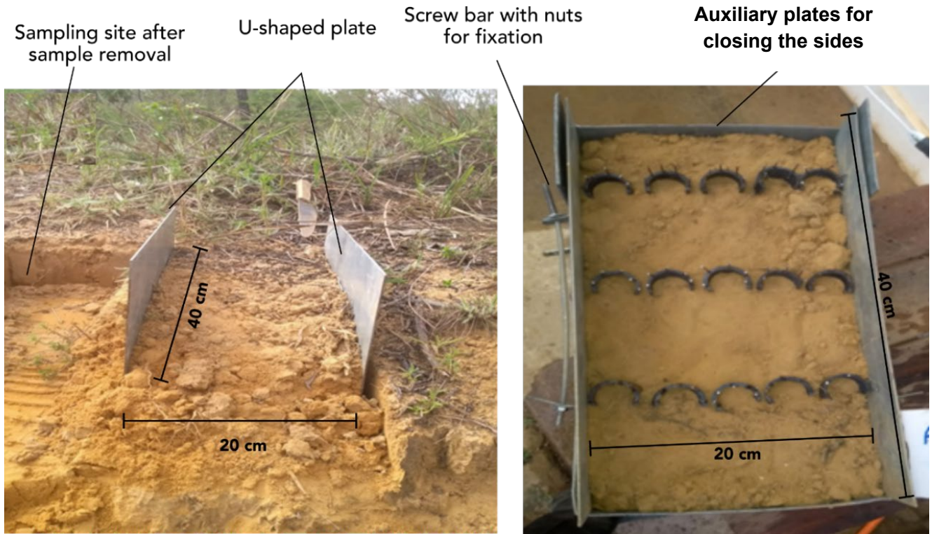
Figure 4 – (A) Soil sample collection with U-shaped plate and (B) soil sample prepared for evaluation.
