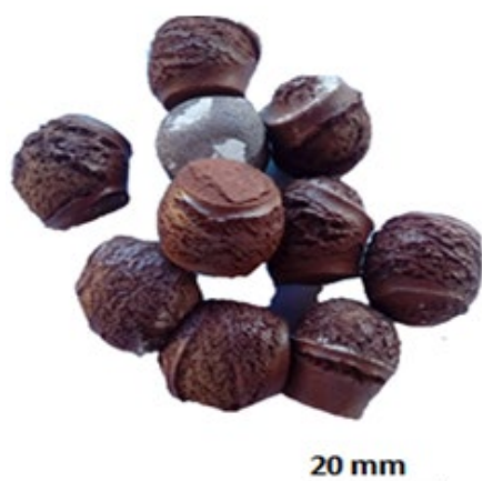
Figure 6 – Photo of the artificial lightweight aggregates clay produced.
